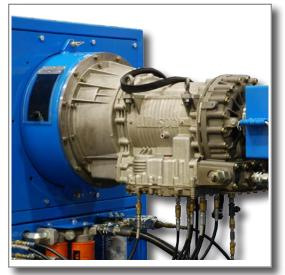
Enclosed indexing assembly allows for safe, rapid rotation of transmission under test. Power indexing available.
