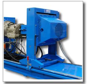
The eddy current absorber can be maneuvered horizontally and vertically and locks into position.
